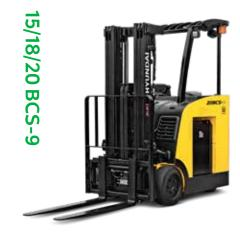
Stand Up Counter Balance Forklift 3,000 - 4,000 lbs. capacity · Cushion Tire
