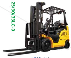
LPG Forklift 5,000 - 6,500 lbs. capacity · Pneumatic Tire
