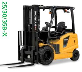
Four Wheel Forklift 48V 5,000 - 7,000 lbs. capacity · Pneumatic TIre
