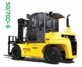
Diesel Forklift 11,000 - 15,500 lbs. capacity
