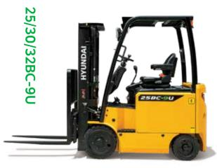
Four Wheel Forklift 36V/48V 5,000 - 6,000 lbs. capacity · Cushion Tire
