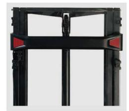
Wide mast provides perfect observation of forks, the field of view is clear and not interrupted by mast sections, cylinder or chains.
