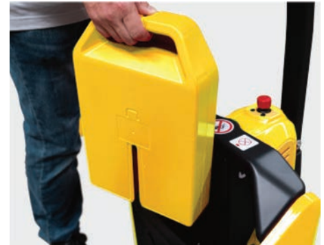
Light weight high quality Lithium battery for easy replacement .
